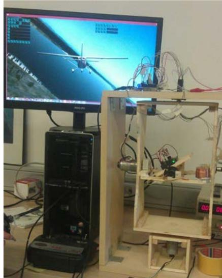
Figure-9 HIL Test Platform and Xplane Simulations
