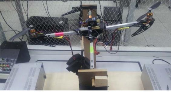
Fig. 3. Experimental Quadrotor Test Platform
