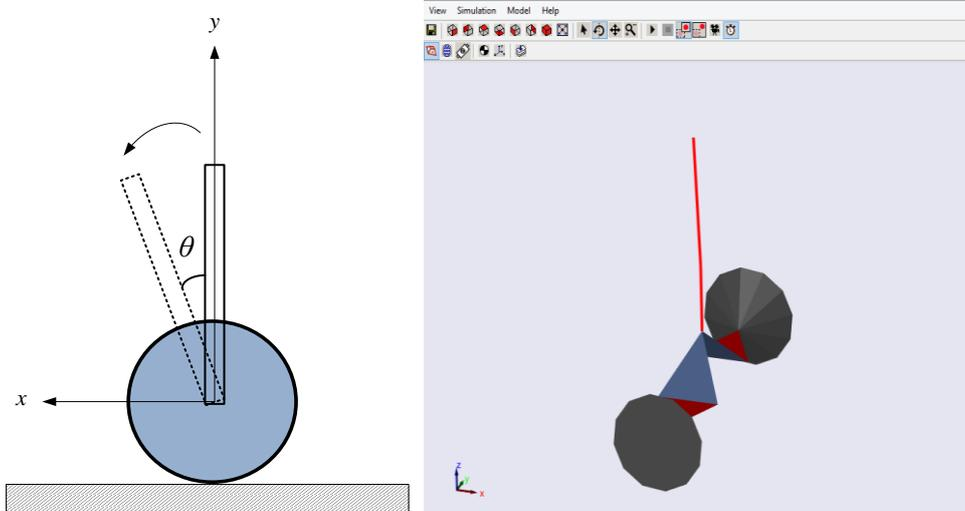
Fig. 1. Model (a) and Simmechanics (b) construction of robot arm on two wheeled moving platform
