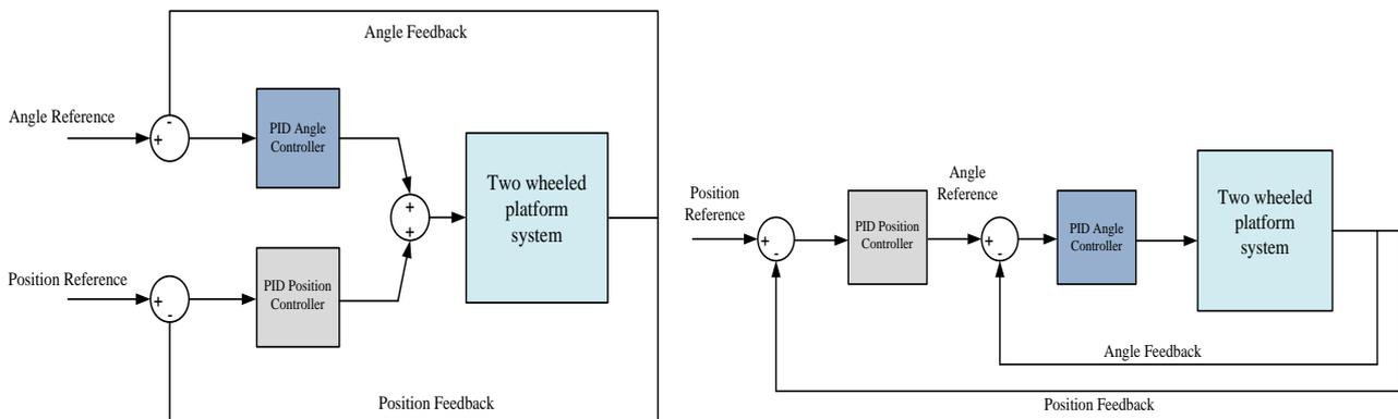
Fig. 2. Parallel PID structure and Cascaded PID structure
