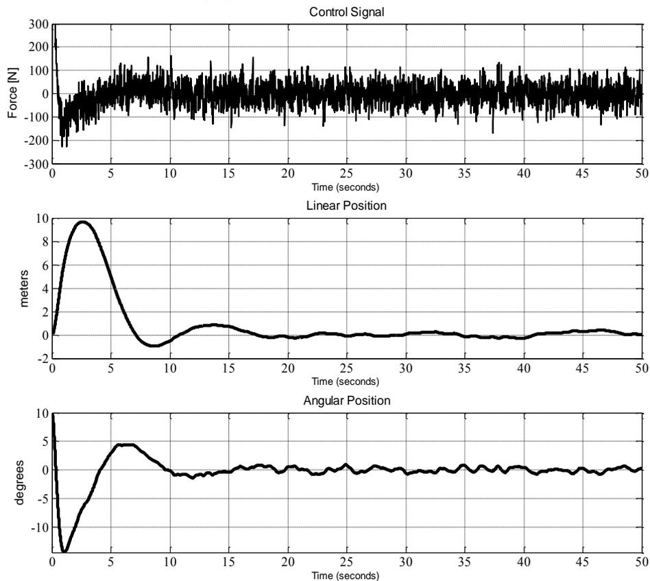
Fig. 5. Control signal and tracking results for LQG control scheme
