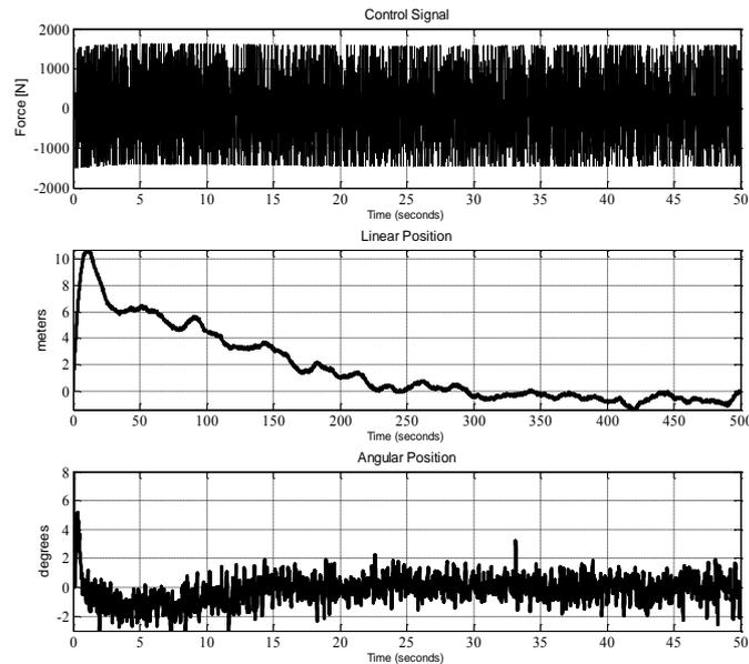
Fig. 3. Control signal and tracking results for parallel PID control scheme
