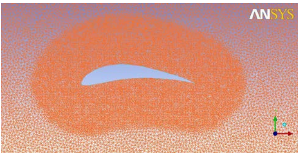
Fig. 3. Mesh structure around Eppler 420 airfoil for CFD analysis
