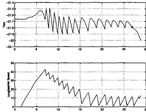
**Figure 12:** The time responses of yaw rate and longitudinal velocity of the vehicle using hysteresis
