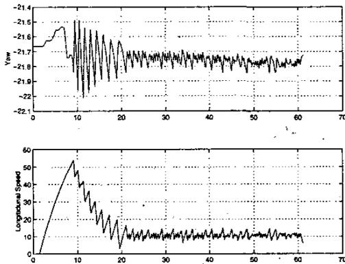
Figure 6: The time responses of yaw rate and longitudinal velocity of the vehicle
