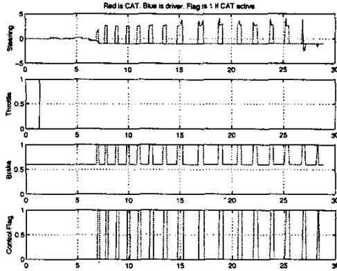
**Figure 11:** Steering wheel angle, throttle, brake commands to the actuators and CAT flag using hysteresis
