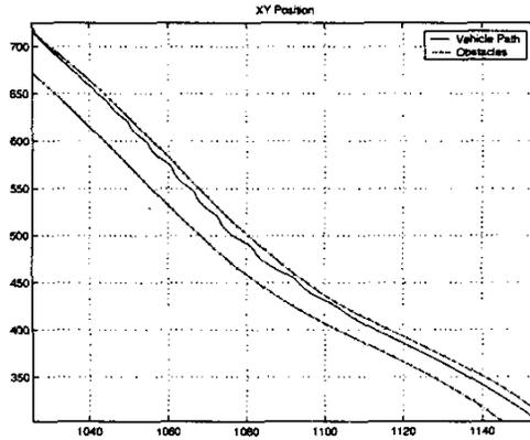
**Figure 13:** The longitudinal and lateral displacements of the vehicle and the obstacles placed on the lane borders using hysteresis
