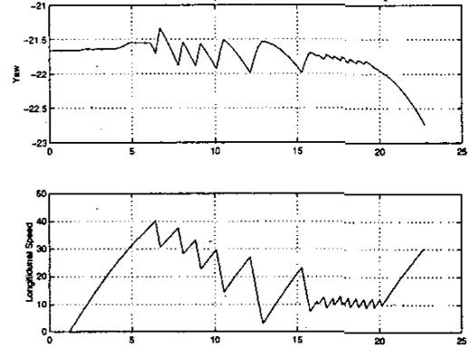
Figure 9: The time responses of yaw rate and longitudinal velocity of the vehicle using dwell-time
