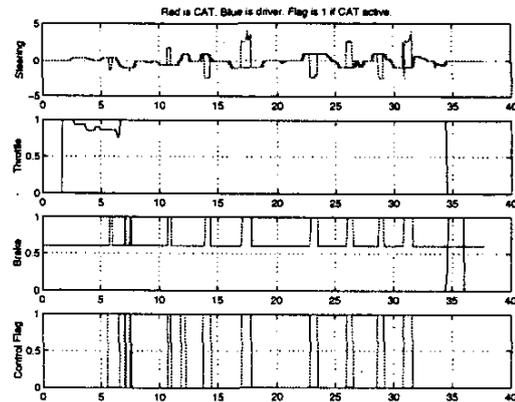
Figure 2: Steering wheel angle, throttle, brake commands to the actuators and CAT flag
