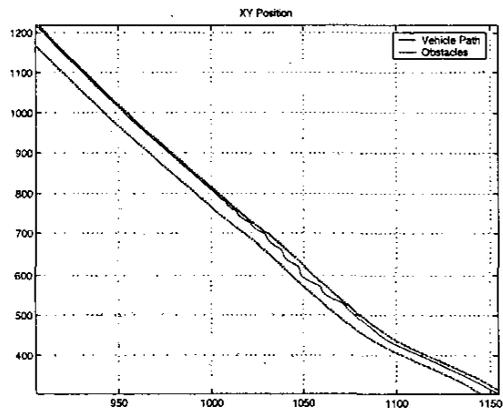
Figure 7: The longitudinal and lateral displacements of the vehicle and the obstacles placed on the lane borders
