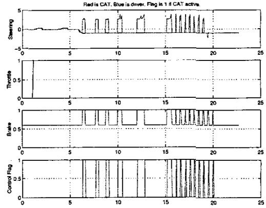
Figure 8: Steering wheel angle, throttle, brake commands to the actuators and CAT flag using dwell-time
