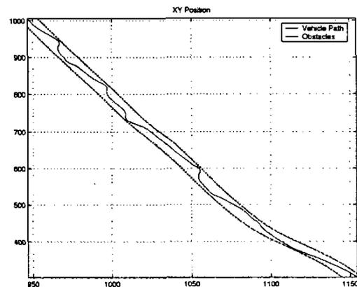
Figure 4: The longitudinal and lateral displacements of the vehicle and the obstacles placed on the lane borders
